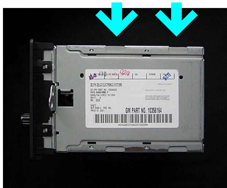
Figure 1: Place the radio on a stable work surface – the front of the radio to your left and the bottom of the radio facing up. Remove the bottom plate carefully with a flat head screwdriver. Around the rim of the bottom plate on the sides are small beaded lock points – 2 on each of the three sides (↑). Begin at the one at the top left of the radio (A) by prying the head of the screwdriver under the plate (see picture below) and twisting slightly and leveraging up until the plate comes loose. Repeat the steps on one of the lock points on the back of the radio (B) – usually only two or three are required till the bottom plate springs free exposing the bottom of the radio circuit board.
