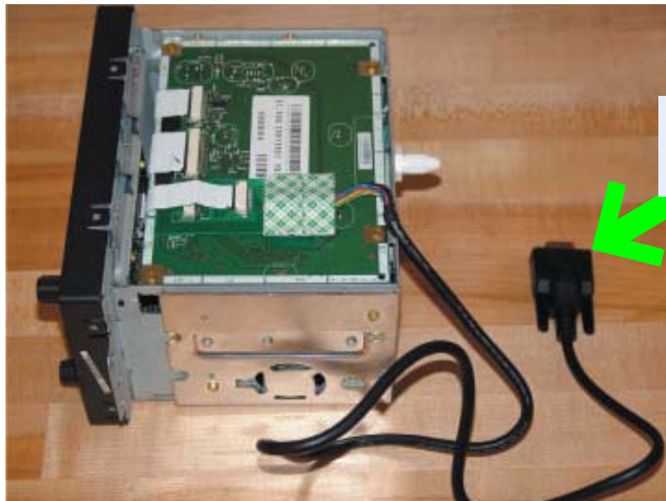
Figure 9: The completed interface connection – now plug connector A to the RGB interface referred to on Page 1. The radio is then ready to return to the dash of the vehicle.
