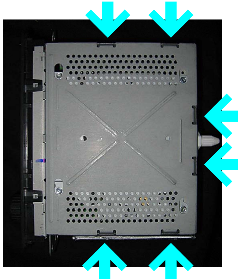
Figure 1: Place the radio on a stable work surface – the front of the radio to your left and the bottom of the radio facing up. Remove the bottom plate carefully with a flat head screwdriver. Around the rim of the bottom plate on the sides are small beaded lock points – 2 on each of the three sides (↑). Begin at the one at the top left of the radio (A) by prying the head of the screwdriver under the plate (see picture below) and twisting slightly and leveraging up until the plate comes loose. Repeat the steps on one of the lock points on the back of the radio (B) – usually only two or three are required till the bottom plate springs free exposing the bottom of the radio circuit board.
